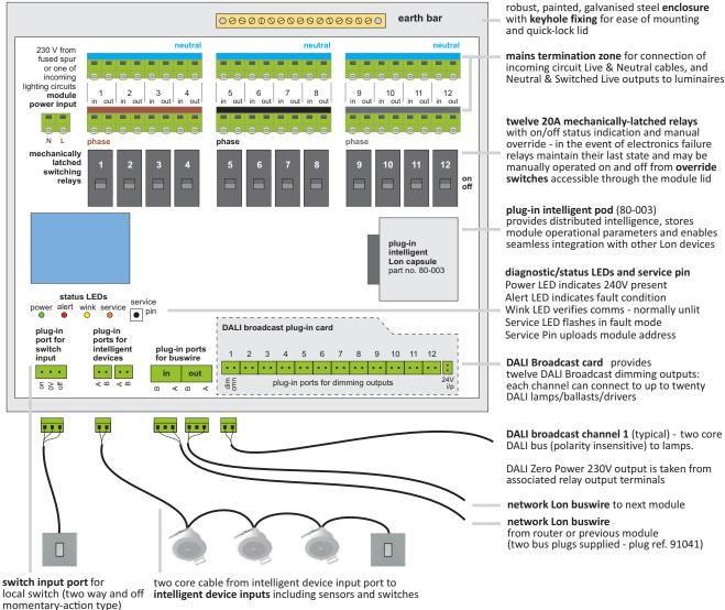
Module supplied with three-pin plug ref. 91043.
